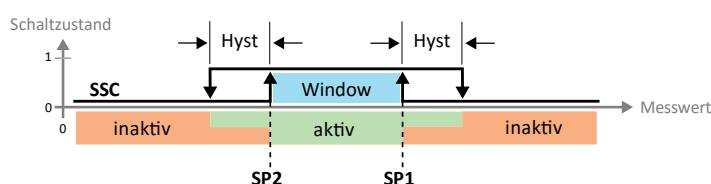
In window mode, the switching points SP1 and SP2 are set for the switching output. The switching window (range between SP1 and SP2) and the hysteresis must be within the detection range.
