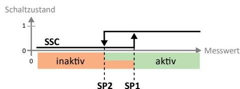
The switching behaviour is defined via a switch-on point SP1 and a switch-off point SP2. If the measured value increases, the switching output is inactive as long as the measured value is between the start of the detection range and the switch-on point SP1. If the measured value increases above the switch-on point SP1, the switching output becomes active.
