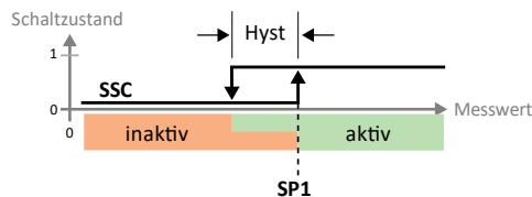
The switching behaviour is defined via a limit value SP1 and a hysteresis. The hysteresis must be within the detection range.
