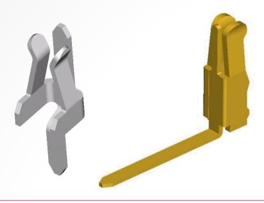
M20 and M22 sockets feature dual beam contacts, typically in phosphor bronze or other high-quality spring material. The dual beam connection gives good durability, repeatable retention and a reliable connection, offering a dependable, cost-effective connector. Design types include flat beam designs (as shown above) and tuning fork designs.
