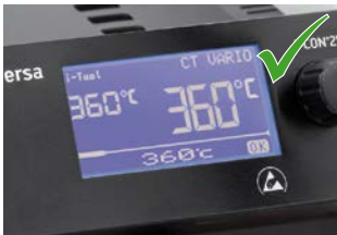
340 – 360 °C for lead-free solder
