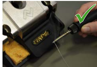
Add new solder after cleaning
