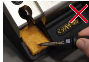
DAMP – NOT WET!
