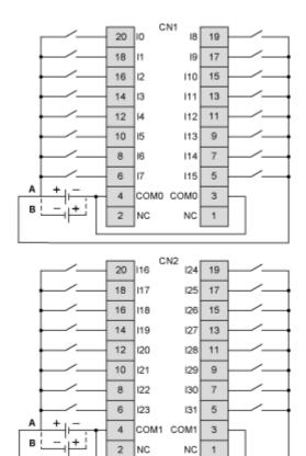
The COM0 and COM1 terminals are not connected internally
