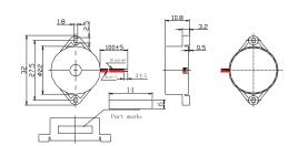
Dimensions : Millimetres Tolerance: ±0.5mm
