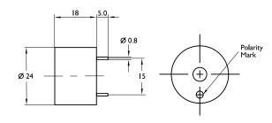
Dimensions : Millimetres Tolerance: ±0.5mm
