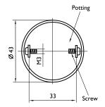
Dimensions : Millimetres Tolerance: ±0.5mm
