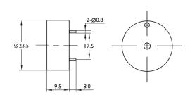
Dimensions : Millimetres Tolerance: ±0.5mm
