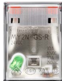
Relay with DC Coil (LED: Green)
