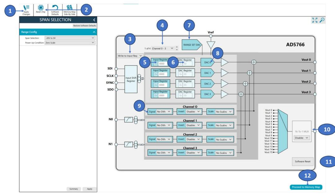
Figure 8. Main Window for the EVAL-AD5766ARDZ ACE Software
