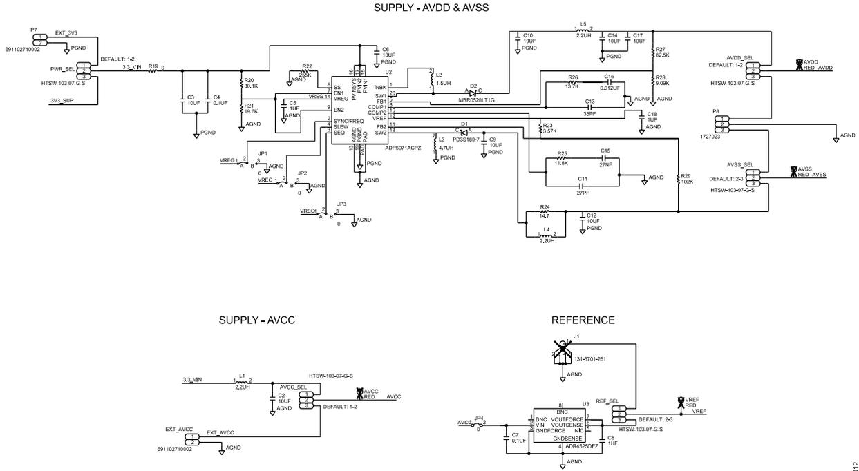
Figure 11. ADP5071 Power Solution, AV<sub>CC</sub>, AV<sub>DD</sub>, AV<sub>SS</sub>, and Reference Power Supply Selection
