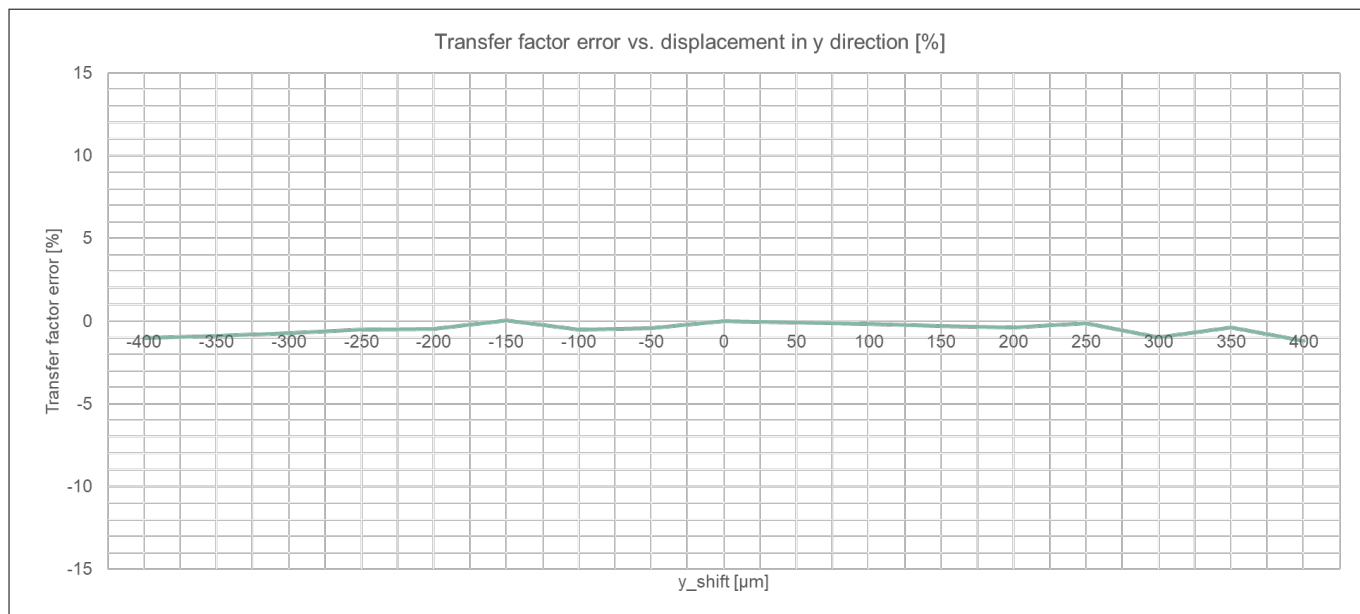
Figure 16 Transfer factor error due to sensor displacement in y direction
