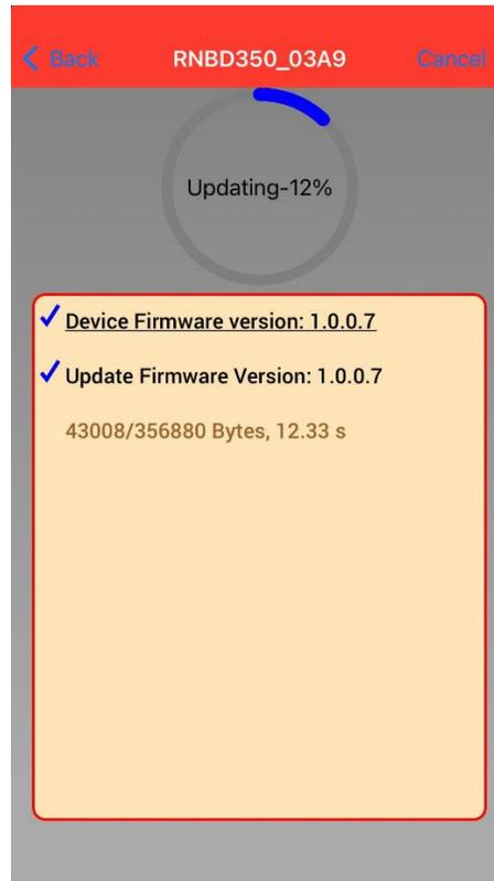
Figure 8-31. Microchip RNBD Utility Tool OTA DFU Firmware Image Receive in Progress
