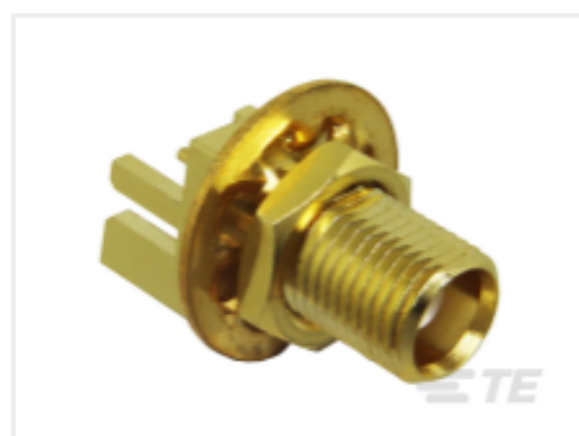
TE Part # L9000245-01 MCX Jack 50 Ohm .031 PCB Edge Mount
