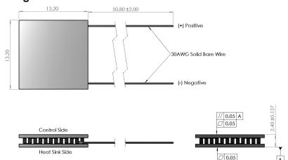
Ceramic Material: Al<sup>2</sup>O<sup>3</sup> / Solder Construction: 232°C, SbSn
