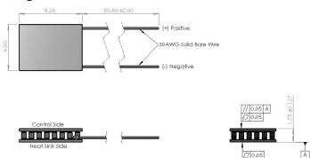
Ceramic Material: Al<sup>2</sup>O<sup>3</sup> / Solder Construction: 232°C, SbSn
