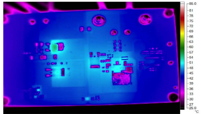
Figure 6. Thermal Map, Backside at 12V IN and 1.5A OUT (T A = 25°C)
