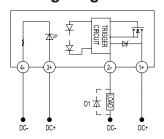
Note: When the relay is used for inductive load control, please be sure to use a suppression circuit, just like the drawing above. Both load terminals are inverse paralleled with a fly-wheel diode D1.
