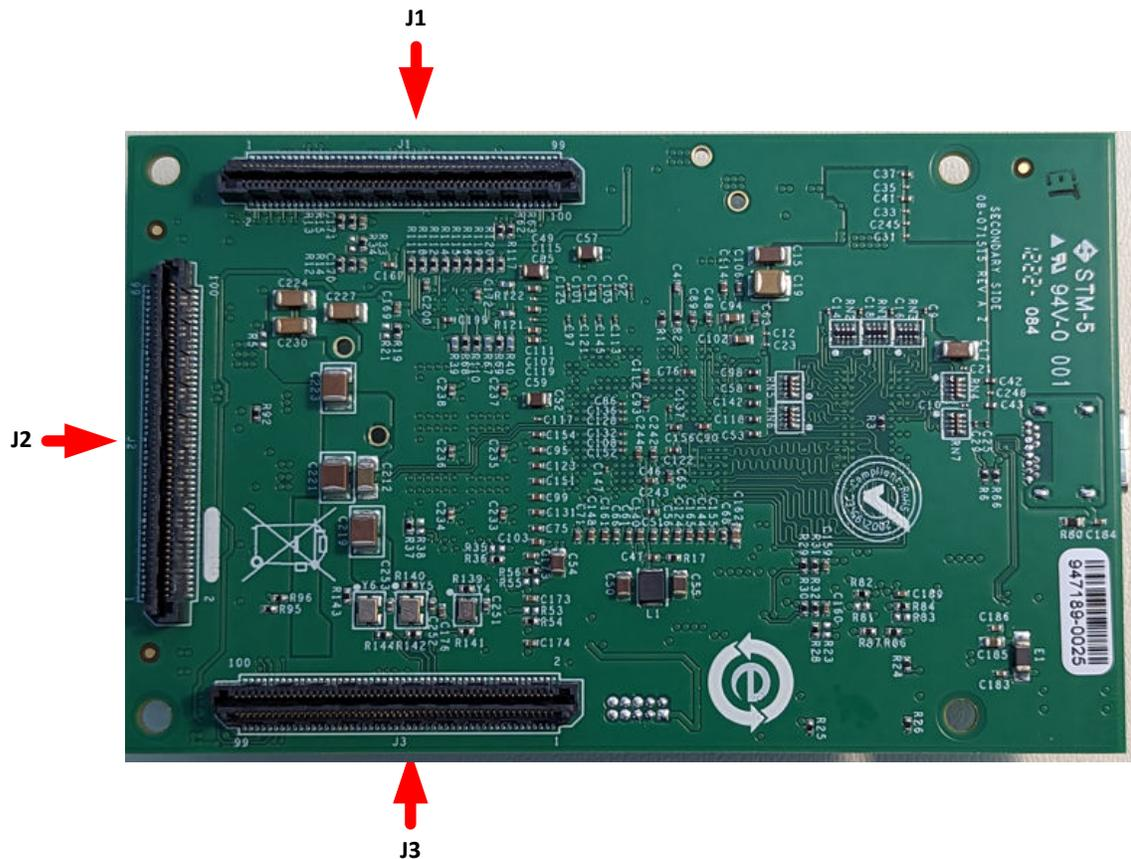
Figure 3-9: Connector Locations Bottom View
