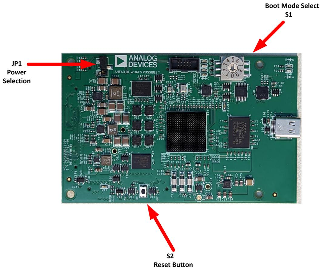
Figure 3-6: Switch/Jumper Locations
