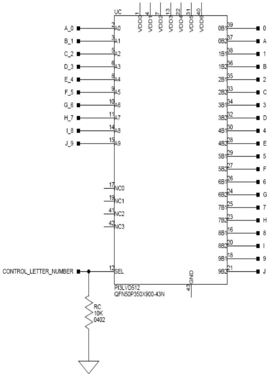
Figure 3-4: Example of a Bus Switch
