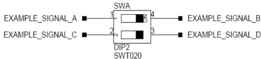
Figure 3-3: Example of a Mechanical Switch (Equivalent to Example of Individual FET Switches Figure)
