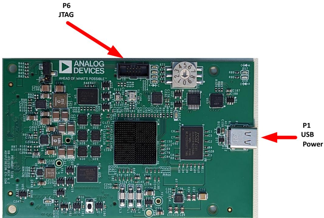
Figure 3-8: Connector Locations Top View
