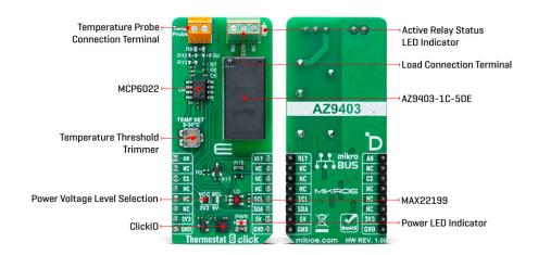
The probe detects real-time temperature changes, while the trimmer allows users to define a threshold temperature level. By comparing the probe's readings to the set threshold, the board activates or deactivates its relay, the AZ9403-1C-5DE SPDT from Zettler, enabling precise and automated control of external devices based on temperature conditions. The temperature limit set by the onboard trimmer can be monitored as an analog voltage output through the AN pin of the mikroBUS™ socket.
