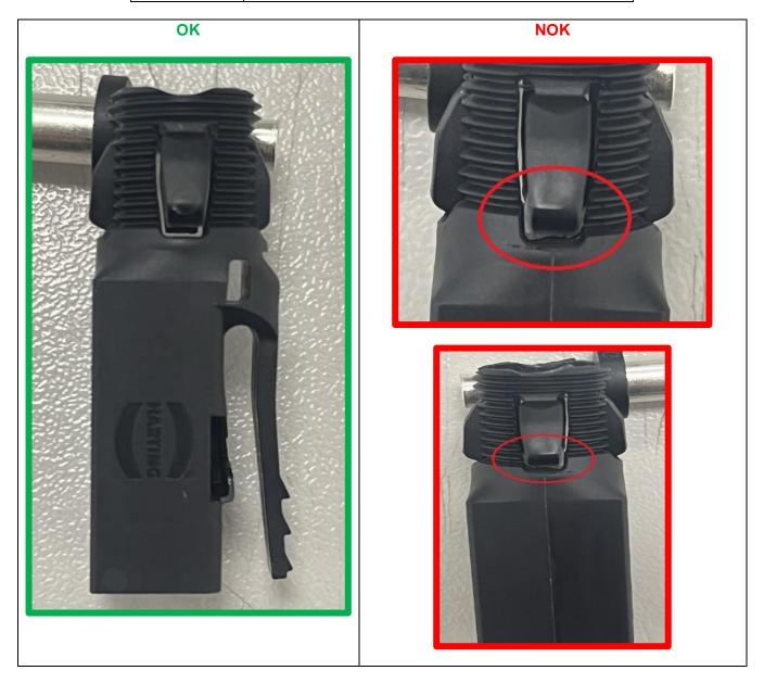
If you received parts that have a burr on the fixing clips, they should be returned to HARTING. For return orders, please contact your HARTING customer service representative and identify that you have product to return, and the concern will be addressed with replacement parts as needed.
