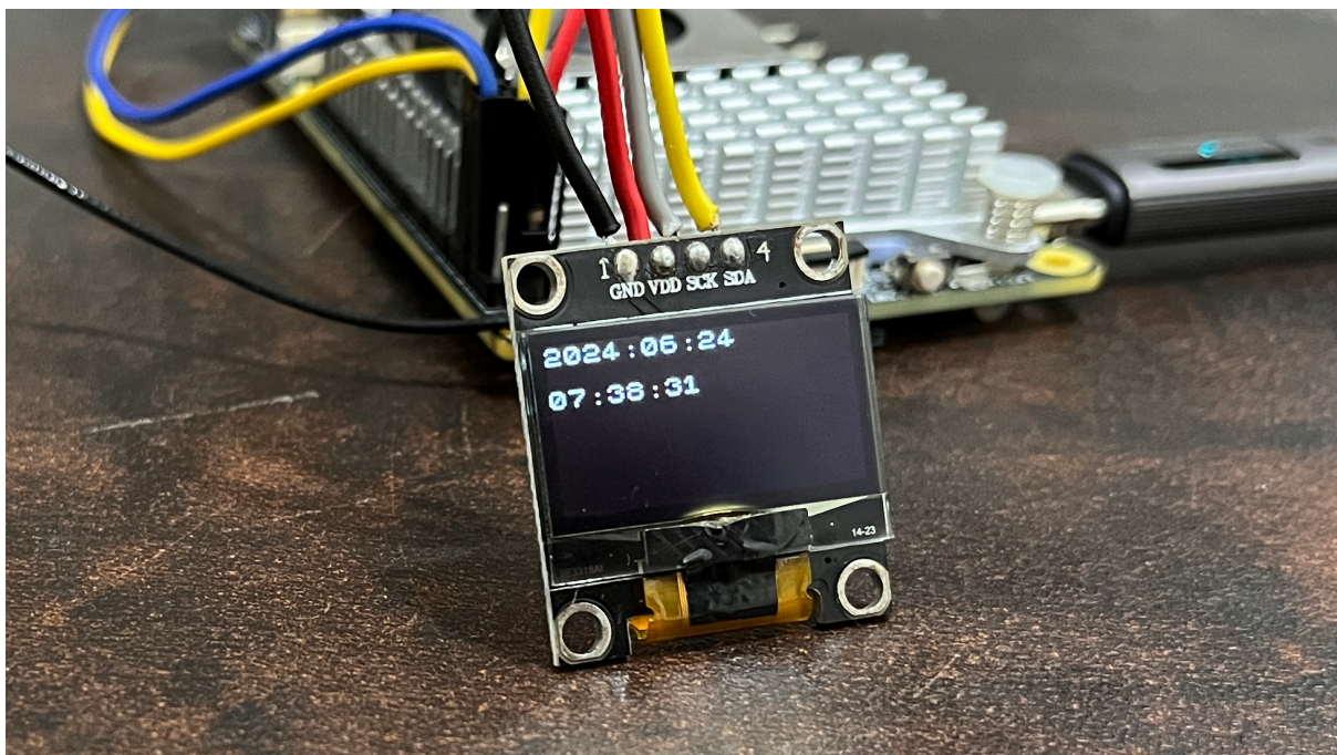
Fig. 5.23: Date & Time on 128x64 OLED
