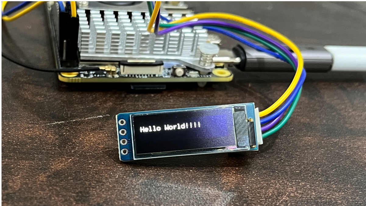
Fig. 5.22: Hello World!!!! on 128x32 OLED
