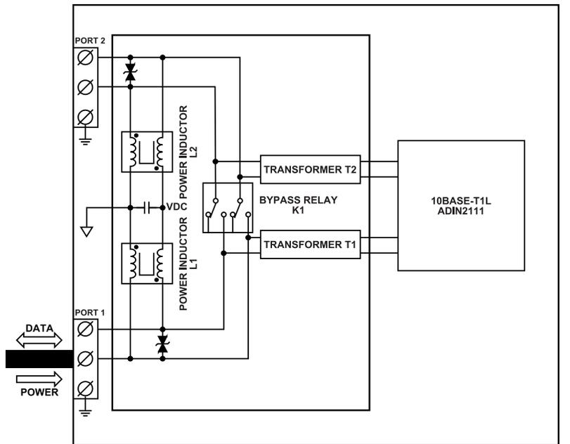
Figure 7. Power Forwarding in a Daisy-Chain Network
