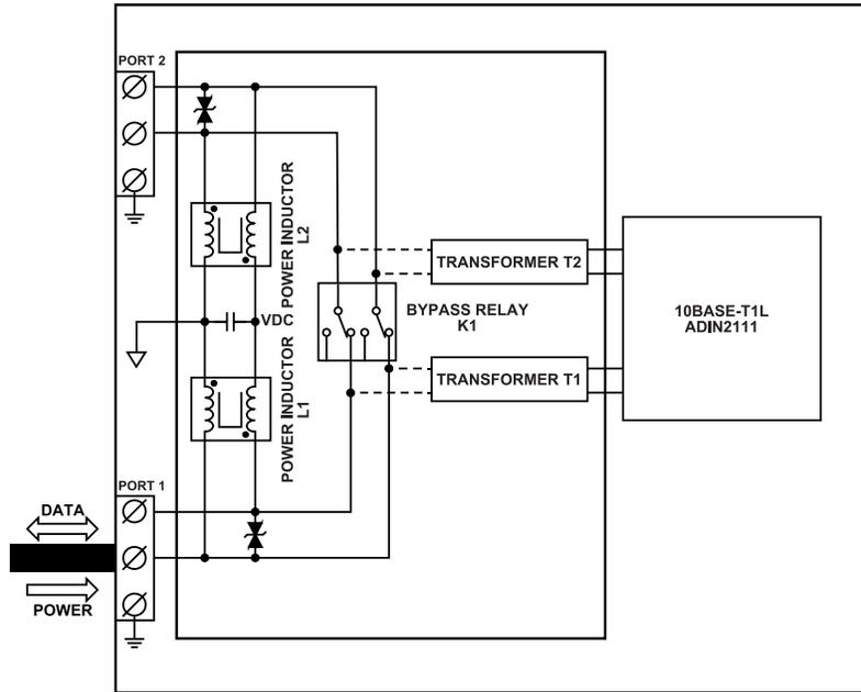
Figure 8. Bypass Relay Circuitry
