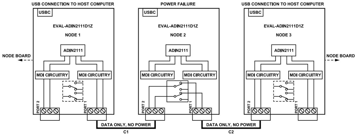
Figure 6. Block Diagram Showing Data Bypass Solution
