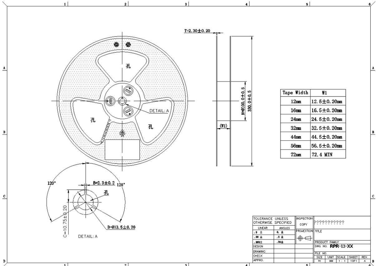
Figure 8: DWM1001 Tape and Reel Dimensions
