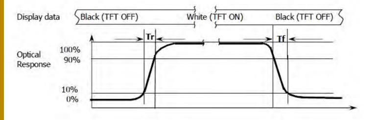
Note (4): Definition of optical measurement setup
