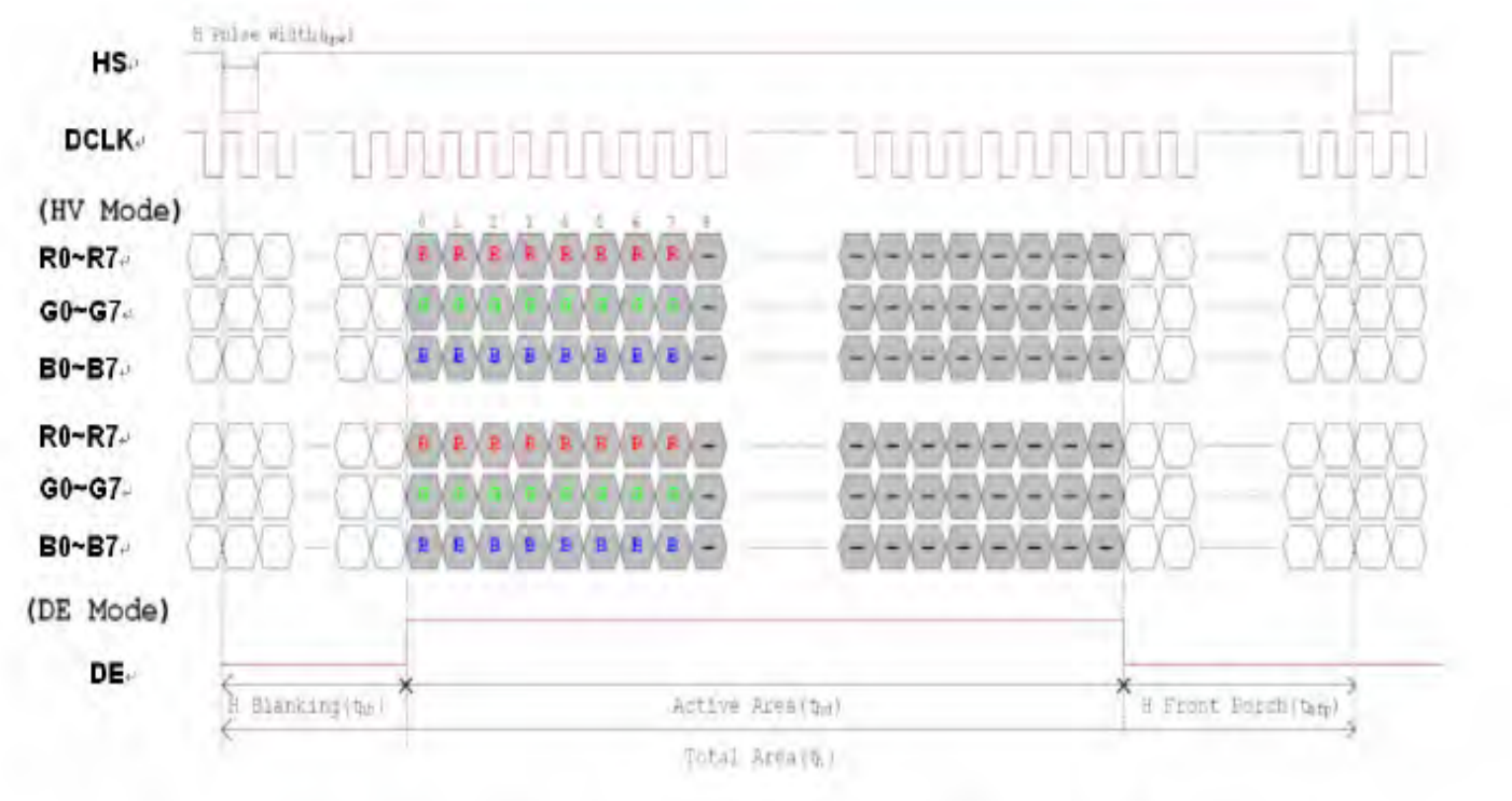
Figure 3. 1 Horizontal input timing diagram.
