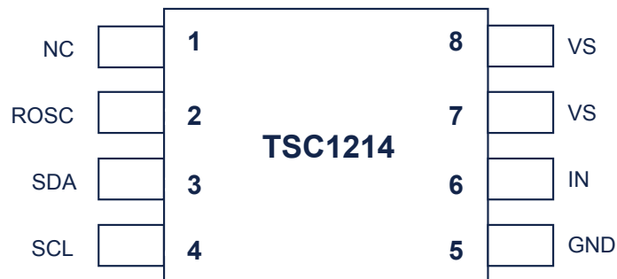
Figure 2. Pin connections (top view)
