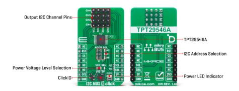
I2C MUX 8 Click communicates with MCU using the standard I2C 2-Wire interface that supports Standard-Mode (100 kHz) and Fast-Mode (400 kHz) operation. The TPT29546A has a 7-bit I2C address with the first five MSBs fixed to 1110. The address pins A0, A1, and A2, are programmed by the user and determine the value of the last three LSBs of the I2C address, which can be selected by onboard SMD jumpers labeled as ADDR SEL, allowing selection of the I2C address LSBs.
