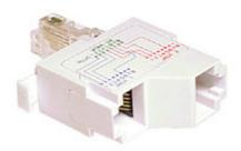
Cat-5E splitters enable 2 different devices to share the same cable and outlet. They are usually used in pairs, one at the outlet and one at the patch panel. Narrow design is ideal for high-density patch panels because the two sockets are mounted vertically to avoid blocking neighbouring sockets. Several standard wiring variants are available. Colour is white. A Data/Data Splitter with a short (100mm) cord is also available.
